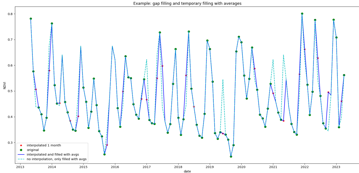
Figure 12: Example of gap filling. Green points are the original time series. Red stars show linear interpolation for gaps up to one month. The dark blue line shows the trend created with the original data, one month interpolation, and remaining gaps filled with averages. The cyan dotted line shows the trend if all gaps were filled with the monthly averages, indicating places where linear filling could cover up the seasonal shape. Filling one month was found to be the best compromise between maintaining enough data for recovery rate calculation while not overly smoothing the dataset.
